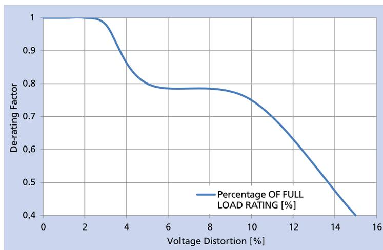
This plot assists in proper de-rating of a Matrix AP Harmonic Filter in environments with a given voltage distortion. Example: In a system with 10% voltage distortion, a Matrix filter will need to be oversized by 25% to obtain the same performance as an appropriate filter in a 0% distortion environment.
