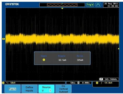
Figure 8: Ripple/Noise diagram of measurement results
