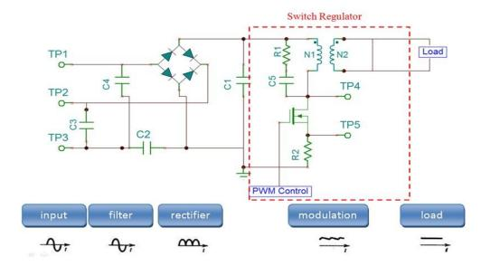
Figure 1: SMPS circuit diagram
