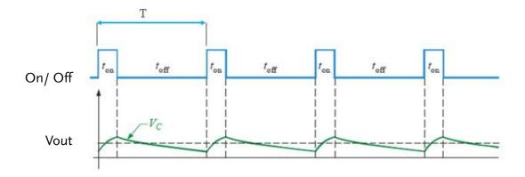
Figure 2: SMPS voltage at the switch and at the regulated voltage output
