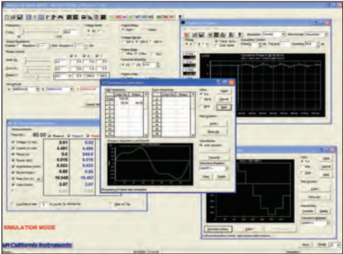
Harmonically distorted waveform.
