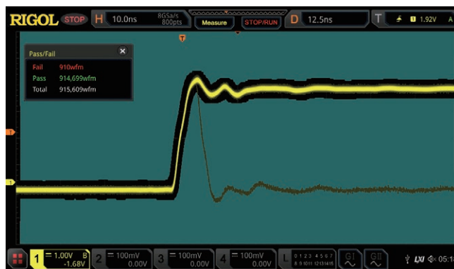
The Pass/Fail test function can quickly make statistics on the occurrence probability of the signal exceptions.
