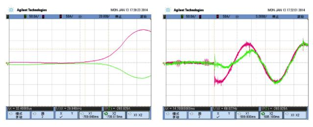
The SVG recalculates the required load accurately and quickly. The IGBT technology switches with high speed, quickly matching the load requirement.
