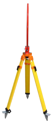
HLA 6121, mounted on tripod CTP 6099, Y position
