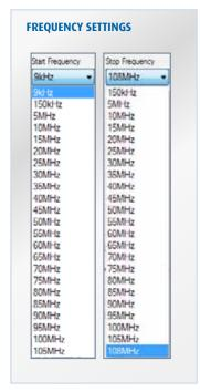
**FFT 3018 EMI Receiver** is ideal for conducted emission measurements from 9 kHz to 108 MHz according to CISPR 25 Standard.
