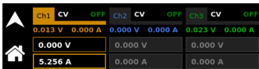
Figure 3-10: DASHBOARD Screen Current Selection-Field Active using Encoder switch
