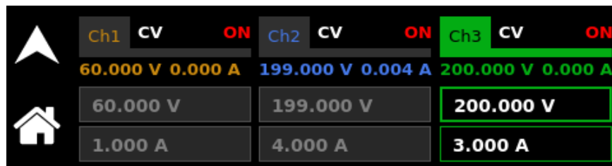
Figure 3-26: Real-Time, Immediate Output Parameter Adjustment
