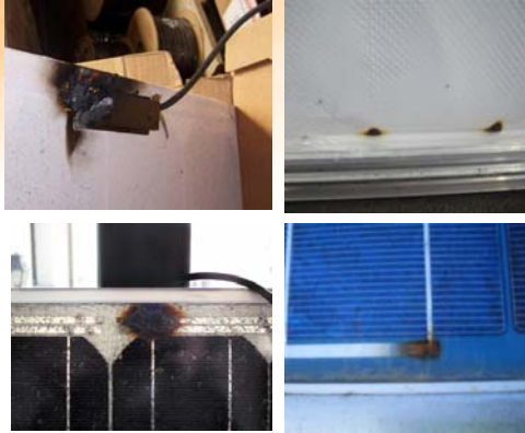
Arcing in PV DC-Arrays
