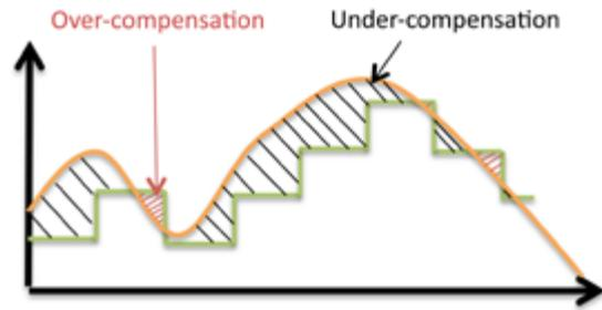
Traditional capacitor type PFC systems take 20ms-40s to respond to a change in load. Their delay combined with the stepped response performance means that they are perpetually over or under compensating.
